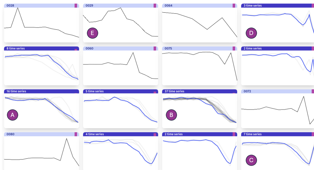
Figure 12. In this example from the welding use case scenario, the majority of data comprise welds that visualize expected behavior (A and B). Other, smaller clusters visualize patterns with a peak toward the end, with differences in the timing of these peaks (C and D), indicating differences in the end phase of the welding process. Our tool can also easily detect individual welds that are anomalous, such as depicted in E.
